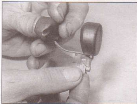
10.8a Hook the needle valve onto the tab ...
