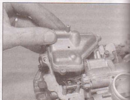
10.10b ... and install the float chamber
