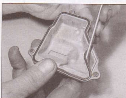
10.10a Fit a new gasket into the groove ...
